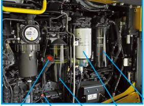
Engine oil fill Fuel filter Oil filter
